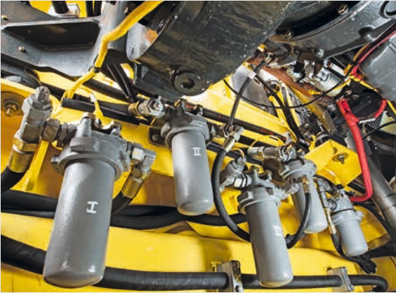
Filter system in the hydraulics.
