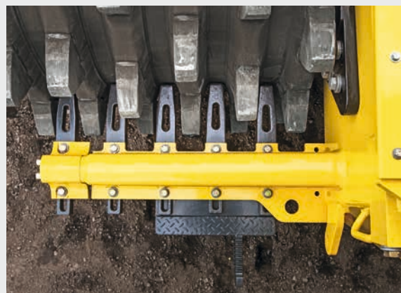
Clean wheels with double-acting scrapers for optimum compaction.
