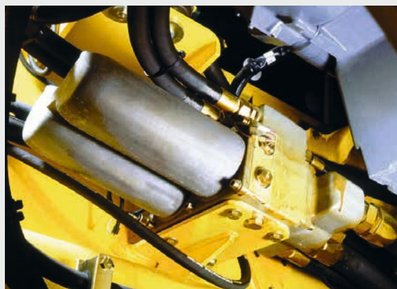
Electronically monitored hydraulics return flow filter system.
