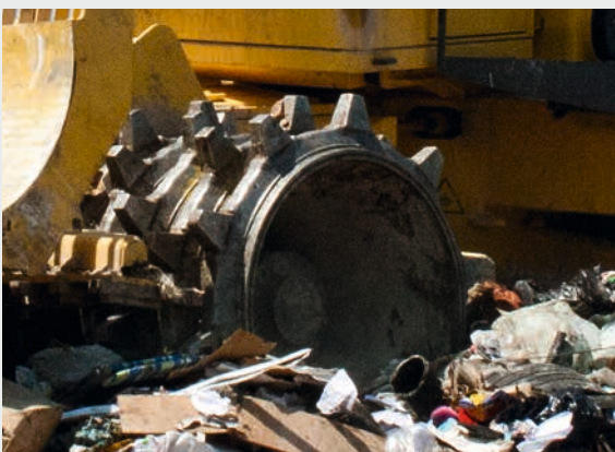
Scrapers ensure clean wheels and guarantee high compaction.
