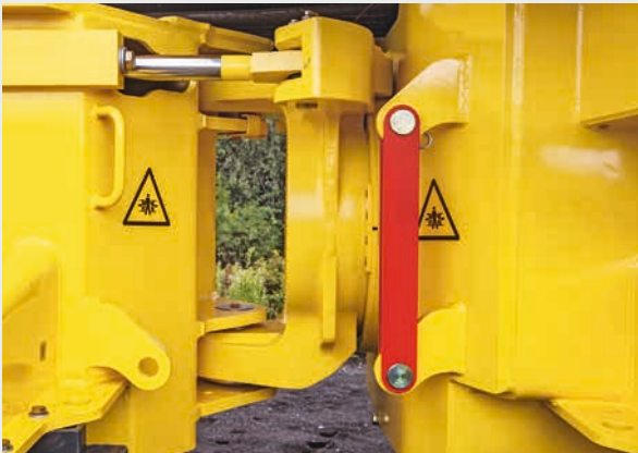
Optimum traction: the oscillating articulated joint provides continuous ground contact.
