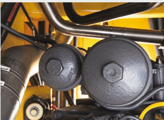
Multi-stage fuel filtering system (shown -4).
