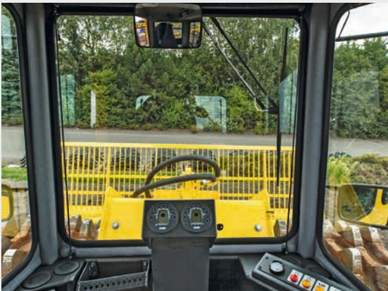
Cab with large glass areas for a clear view over the work in progress (shown -4).
