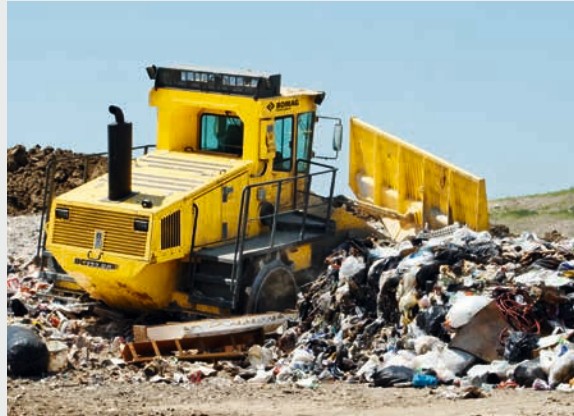
Optimum compaction is achieved by the effect of the oscillating joint, which supplies uniform load distribution to the compactor wheels.
