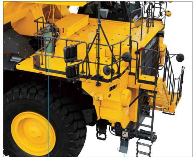
Grease pump and reservoir
