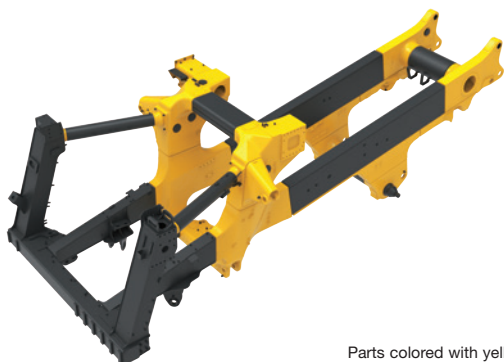
Parts colored with yellow show cast-steel components.
