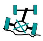
Machine stopped, when lifting mouvements starts (working mode) the axle is blocked and gives rigidness to the chassis.
