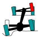
On unlevelled ground according to the position of the center of gravity the machine could be not stable enough or fall down.
