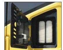
External air conditioner filter
