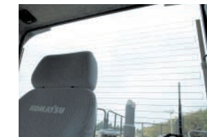
Rear heated glass provides clear view even in freezing or condensation conditions.
