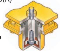
The large cab is mounted with Komatsu's unique ROPS/FOPS viscous mounts. The low-noise engine, hydraulically driven fan, and hydraulic pumps are mounted with rubber cushions, and the cab sealing is improved to provide a quiet, low-vibration, and comfortable operating environment. Pressurization in the cab keeps dirt out, further enhancing the operator's comfort.
