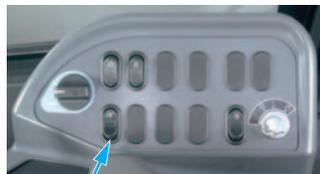
Dual mode engine power selection switch
