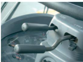
The Komatsu two-lever electronic shift control levers provide easy gear selection and directional changes. The transmission levers can be operated without removing the operator's hand from the steering wheel, allowing improved
