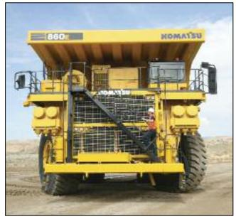
Komatsu's 860E-1K offers stairway access with entry from either the right or left side of the truck depending on the customer's preference.
