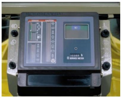
Electronic display and monitoring system continuously monitors all operating systems, keeping the operator well-informed of machine conditions.
