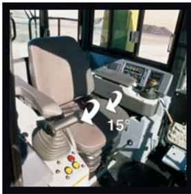
For improved rear visibility during return part of cycle, the operator can adjust seat 15° to the right. The transmission and steering controls move with the seat for best operator comfort.
