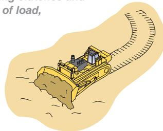
*When dozing downhill, ECMV automatically controls steering clutches and brakes depending on incline of machine or degree of load, reducing counter-steering and producing smooth dozing operation.*
