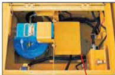
Grease can drum storage location
