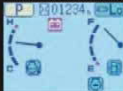
Battery charging abnormal display
