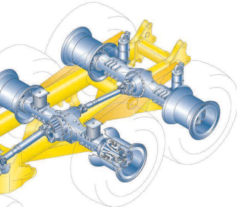
**Hydraulically Controlled Wet Multiple-Disc Brakes and Retarder**
