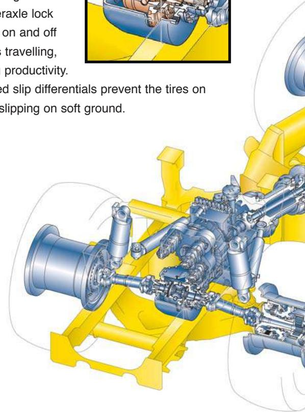
**Hydro-Pneumatic Trailing Arm Suspension**
