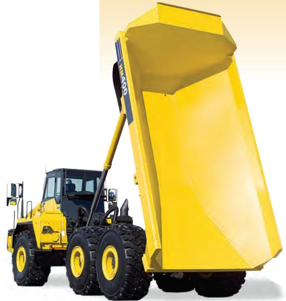
***Interaxle & differential locks provide excellent traction in rough terrain***
